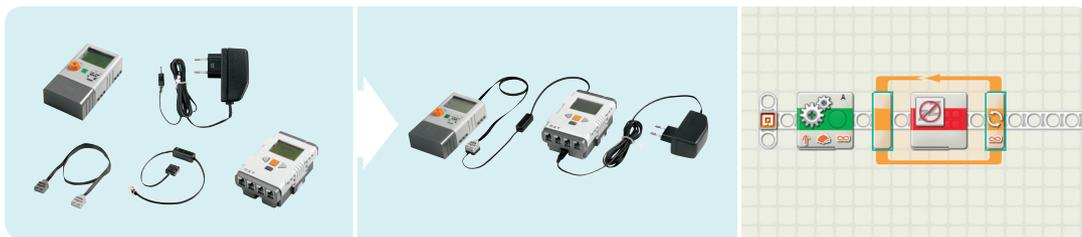
You need to use two different converter cables to connect the LEGO Energy Meter with the LEGO MINDSTORMS NXT, Port A.
