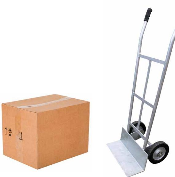
Simple machines have very few parts; compound machines are made up of two or more simple machines. A moving dolly is one example of a compound machine. It has combined two simple machines. The handles are levers that help lift the load, and the wheel and axle help move the load forward easily. The same principle applies to a wheelbarrow.
