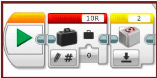
Initialization of variable 10R at 0 and calibration of Gyro Sensor.
