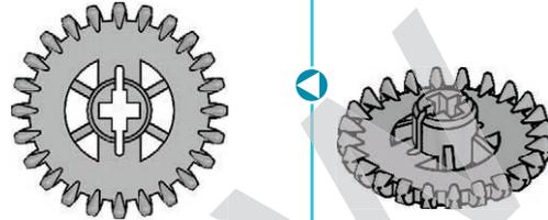
A gear is most commonly defined as a toothed wheel; the teeth of a gear prevent slipping. When one gear is engaged with another gear they are said to mesh. When a set of gears work together they transmit movement and force. A crown gear has special curved teeth that enable it to mesh at right angles with a spur gear. Gears are sometimes categorized as compound machines, but in this material we have included them as simple machines.
