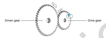
The gear that is closer to the source of power is called the drive gear and the gear that receives power from the drive gear is called the driven gear (or follower gear).
