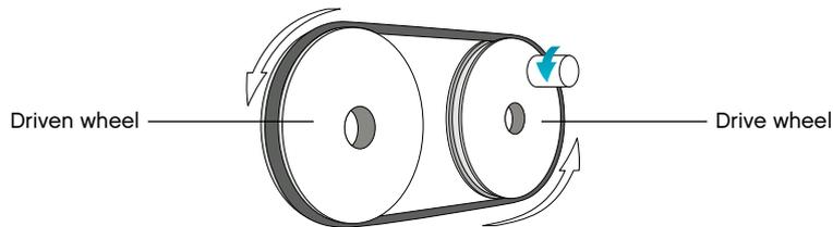
A pulley is most commonly defined as a wheel with a grooved rim for a belt or rope. A belt connecting pulleys can “slip”, meaning that the effort is not being used efficiently. This can happen either when the pulley belt is too loose, or if the pulley wheels differ in size. On the other hand, if the pulley belt is too tight, the belt will create wasteful friction forces on the pulley.
