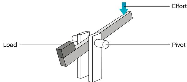
A lever is most commonly defined as a rod or arm that tilts around a pivot, also called a fulcrum, to produce useful motion. The load is moved by the effort (a push or pull) used to make the lever tilt about the pivot. With a lever arm or lever beam, a load can be lifted with the least effort by placing it as close to the pivot as possible, or by applying the effort as far from the pivot as possible.
