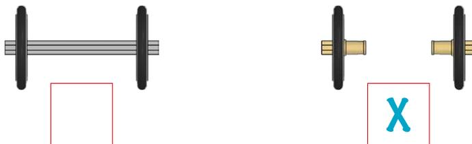
*Model B4 is built with separate axles.*
