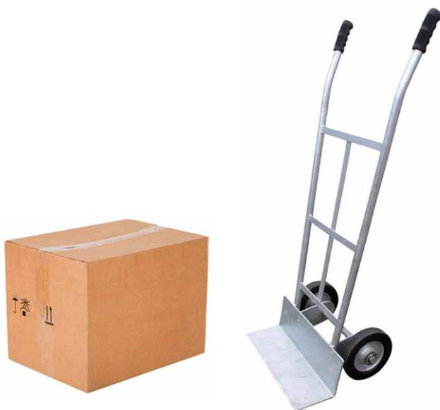
Simple machines have very few parts; compound machines are made up of two or more simple machines. A moving dolly is one example of a compound machine. It has combined two simple machines. The handles are levers that help lift the load, and the wheel and axle help move the load forward easily. The same principle applies to a wheelbarrow.
