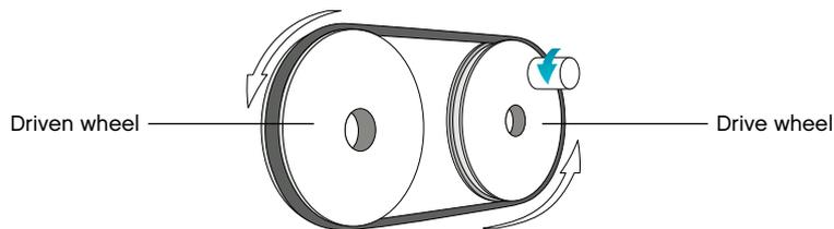
The pulley that is turned by an outside force, such as that from a motor or from a person turning a handle, is called a drive or the drive wheel. When this turns at least one other pulley by a belt, the next pulley is called the driven wheel (or follower).
