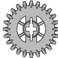
A gear is most commonly defined as a toothed wheel; the teeth of a gear prevent slipping. When one gear is engaged with another gear they are said to mesh. When a set of gears work together they transmit movement and force. A crown gear has special curved teeth that enable it to mesh at right angles with a spur gear. Gears are sometimes categorized as compound machines, but in this material we have included them as simple machines.
