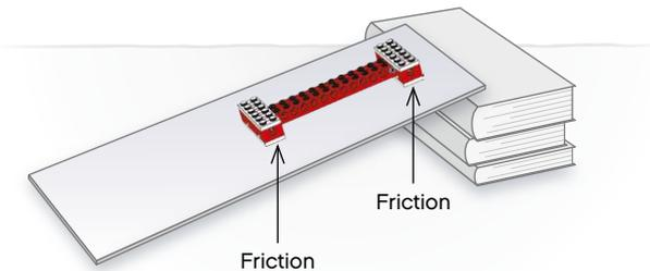
Friction is the resistance met when one surface slides over another; this affects movement (see the “Glossary” section). The effects of friction can be tested using the principle models.
