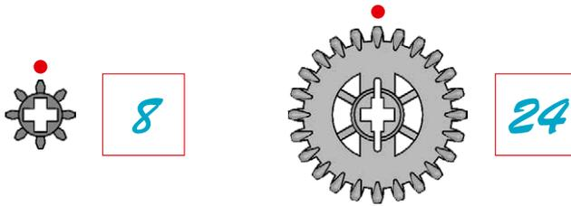
*There are two gears used in model A6: a spur gear (8 teeth) and a crown gear (24 teeth).*
